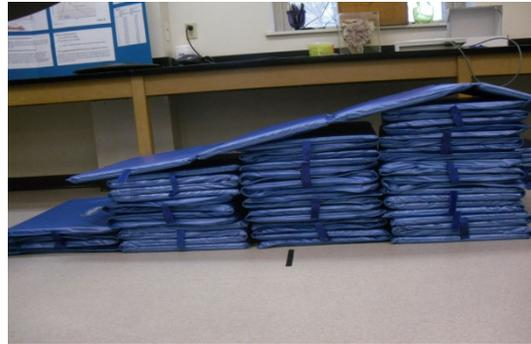
Figure 3. Incline made of Game Craft mats in a 5x4x3 configuration with one mat extended across the top for smoothing.
